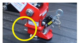
Figure 8: Shift Lock coupler in correct locked position - 1" of the u-bolt stick out
