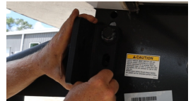
Figure 3: Using existing hardware, install safety chain brackets to Quick Air pin box
