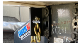
Figure 4: Feed chains into bracket and secure using provided carriage bolts
