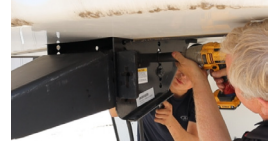
Figure 2: Line up Quick Air pin box and install with original hardware
