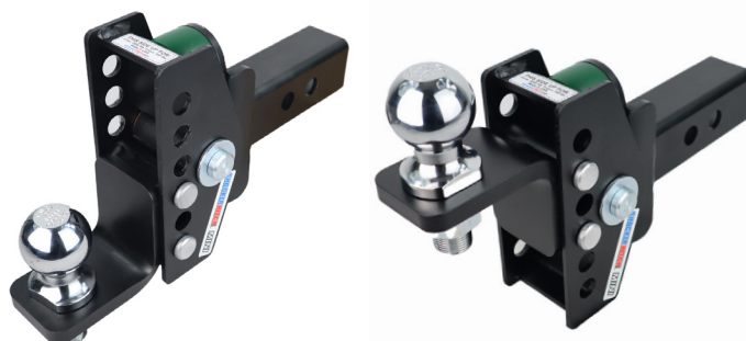
FIGURE 2: GREEN bushings facing "upward" the weight is on the BLACK bushing - 3,500 lb GTW & 350 lbs TW
