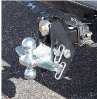
SWAY COMBO BALL: 4" RISE TO 4" DROP 2-5/16" BALL - 20,000 LBS & 2" BALL - 10,000 LBS
