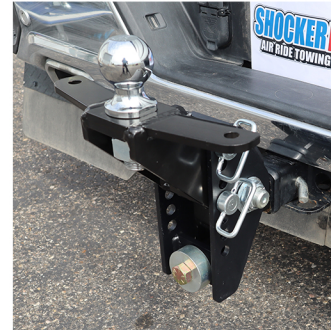
SWAY RAISED BALL: 5" RISE TO 3" DROP 2-5/16" BALL - 20,000 LBS/2" BALL - 10,000 LBS
