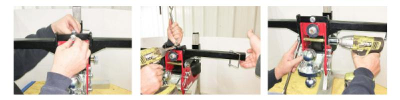
3. Insert 1" x 36" long square tubes in the mounting tube brackets with the plastic endcap out board, adjust to desired width of truck. Install one 5/16" x 1-3/4" flange bolt, washer, and nylock nut through both tubes. *Optional Snapper pins are supplied for quick installation and removal of rubber flaps.*
