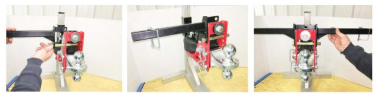
2. Install 7/16" x 1-1/4" flange bolt and nut - support/lift mounting bracket tubes so they are level - final tighten 7/16 bolt - Finish tightening 5/8" x 6" cross bolt.
