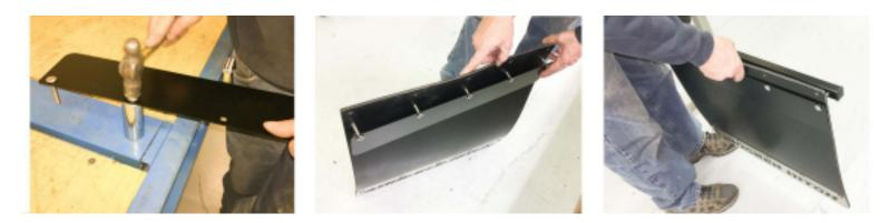
6. Optional Heat Shields are available, these can be installed in a variety of positions to accommodate different exhaust configurations. Install using three existing 5/16 x 2" carriage bolts each side.
