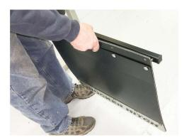
6. Optional Heat Shields are available, these can be installed in a variety of positions to accommodate different exhaust configurations. Install using three existing 5/16 x 2" carriage bolts each side.
