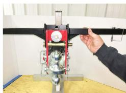
2. Install 7/16" x 1-1/4" flange bolt and nut - support/lift mounting bracket tubes so they are level - final tighten 7/16 bolt - Finish tightening 5/8" x 6" cross bolt.
